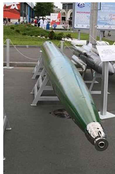
**Russian ShKval super-cavitating torpedo**
